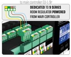
Connecting of wired temperature sensor EU-C-7p
