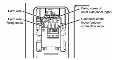
8 Pull the outer side panel (right) towards you while pulling up the fixing tab (1 location) of the powersupply box to disengage the tab.
