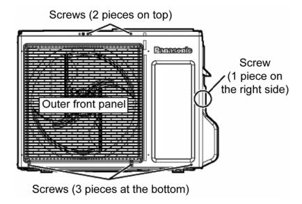
Disengage the tabs on the outer front panel (3 locations on the left side and 1 location on the right side). Remove the outer front panel while pulling it slightly up.
