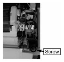
5 Disengage the tabs (3 locations) which fix the electrical component cover (rear) to the power-supply box. Then, remove the electrical component cover (rear) on the right side of the power-supply box.
