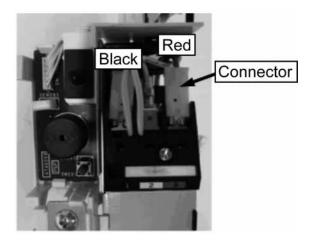
5 Remove the screw (1 piece) which fixes the control board.
