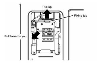
9 Lift up the power-supply box to remove it.
