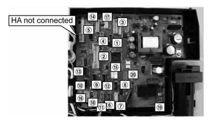
7 Remove the screw (1 piece) of the clamp for the power cord and then remove the clamp.
