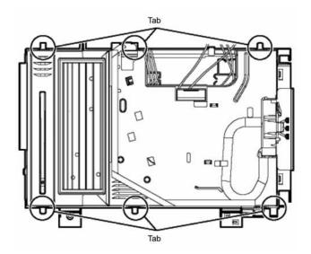
X Notes on disassembly: During the replacement of outdoor control board, the control board and plastic power-supply box are separated by removing the screws (2 pieces) on the soldered surface. These two parts can be replaced as an integrated piece by applying silicon to them.
