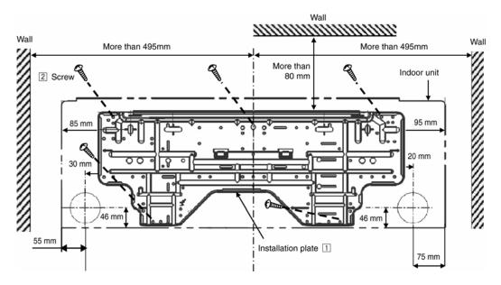
The center of the installation plate should be at more than 495 mm at right and left of the wall. The distance from installation plate edge to ceiling should more than 80 mm.
