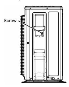
2 Remove the screws (2 pieces) and disengage the tabs (2 locations) of the electrical component cover (terminal plate cover). Then, remove the electrical component cover (terminal plate cover).
