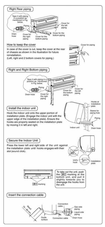
(This can be used for left rear piping and bottom piping also.)
