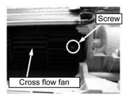
9 Pull out the cross flow fan while lifting up the left side of the heat exchanger.
