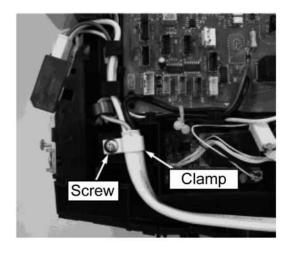
8 Remove the earth wire screw (1 piece) and disconnect the indoor/outdoor connection wires as well as the connector for the white wire connected to the terminal block. Then, remove the control board box.
