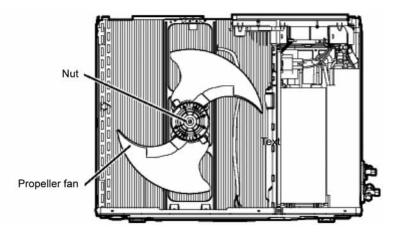
6 Loosen the fixing screws (4 pieces) of the outdoor motor and remove the outdoor motor.
